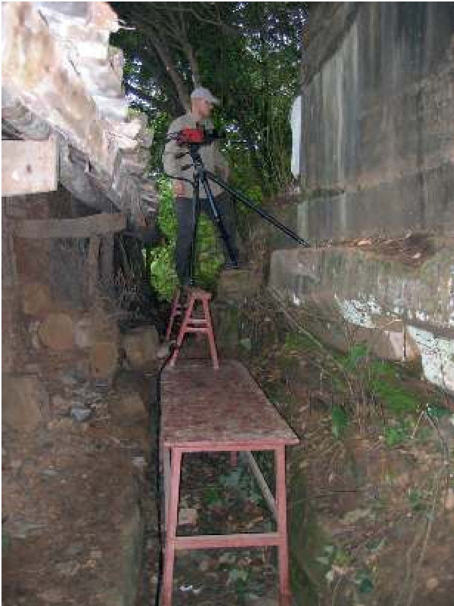
Confined working space I: An engineer from the Institute for Spatial Information and Surveying Technology, University of Applied Sciences Mainz (i3mainz), takes scans of the Diamondsutra at Beishan Monastery; photograph taken in 2009
