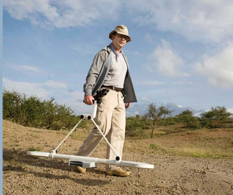
Michael Märker conducting an electromagnetic induction survey at the fossil locality of Makuyuni in northern Tanzania.
