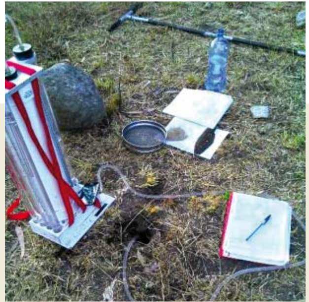
Fig. 9 Measurement of hydraulic conductivity of substrates.
