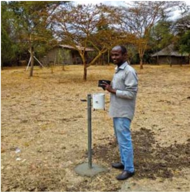
Fig. 8 Rain gauge installed at Melka.
